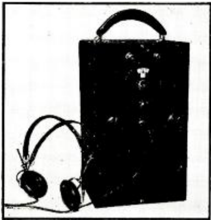
The 2-Tube Superhet., (See Fig. 2 for identification of controls.) with crystal headphones. The tuning range is about 540 to 1,600 kc.
